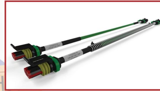
Linear Heat Detection cables have long been the industry standard and provide a continuous heat detection cable run inside the hazard area. Amerex has raised the bar for traditional cable with a more robust abrasion resistant outer jacket and factory installed connectors for reliability and ease of service. The cable is also available with a stainless steel wire protective covering for extreme environments.
