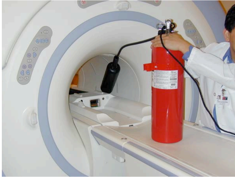
FIGURE 5. Testing the Model 331, 15.0 lb. CO 2 fire extinguisher for magnetic field interactions during exposure to a 3.0-Tesla MR system. While the “tank” showed no magnetic field interactions at 3-Tesla, the “hose” portion was substantially attracted to the 3-Tesla MR system. As such, this may present a serious problem or issue for its use in a 3-Tesla MRI environment.
