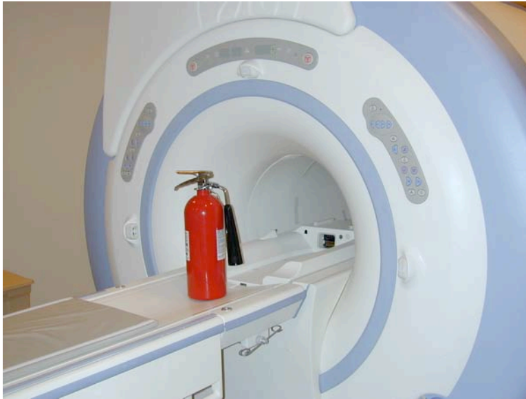
FIGURE 4. Testing the Model 322, 5.0 lb. CO 2 fire extinguisher for magnetic field interactions during exposure to a 3.0-Tesla MR system. Note the lack of magnetic field translational attraction for this fire extinguisher.
