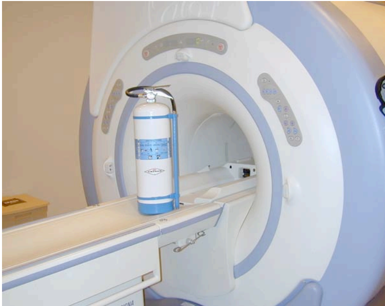
FIGURE 3. Testing the Model B272NM, 2 1/2 gallon Water Mist fire extinguisher for magnetic field interactions during exposure to a 3.0-Tesla MR system. Note the lack of magnetic field translational attraction for this fire extinguisher.
