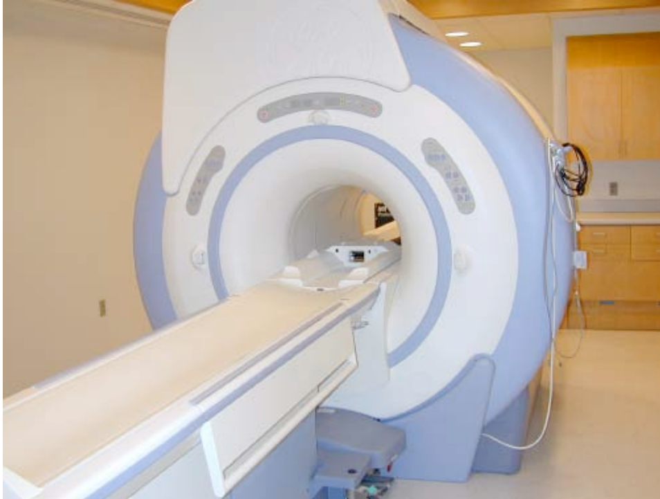
FIGURE 1. The 3.0-Tesla MR system (General Electric Medical Systems, Milwaukee, WI) used for assessment of magnetic field interactions for the four different fire extinguishers from the Amerex Corporation.
