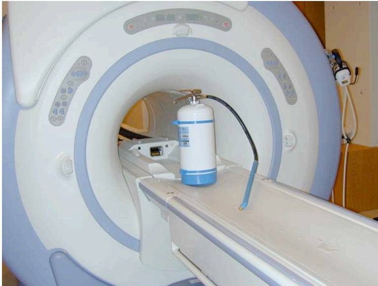
FIGURE 2. Testing the Model B270NM, 1 3/4 gallon Water Mist fire extinguisher for magnetic field interactions during exposure to a 3.0-Tesla MR system. Note the lack of magnetic field translational attraction for this fire extinguisher.
