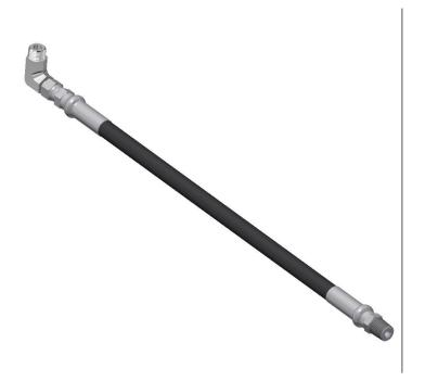
To aid in the installation of systems, an optional Actuation Hose is available. This 16" or 32" hose connects the MRM (Mechanical Release Module), PRM (Pneumatic Release Module), or SRM (STRIKE™ Release Module) actuation port to the top of the Agent Cylinder Discharge Valve(s).
