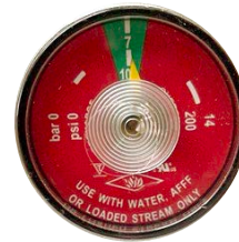
Water Mist Extinguisher Pressure Gauge
