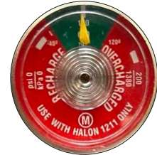
Halon Extinguisher Pressure Gauge
