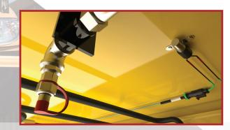
A combination of Linear Heat Detection cable and Spot Heat Detectors provides flexibility in your installs. It also provides rapid heat detection and system activation, which means less damage and less downtime.
